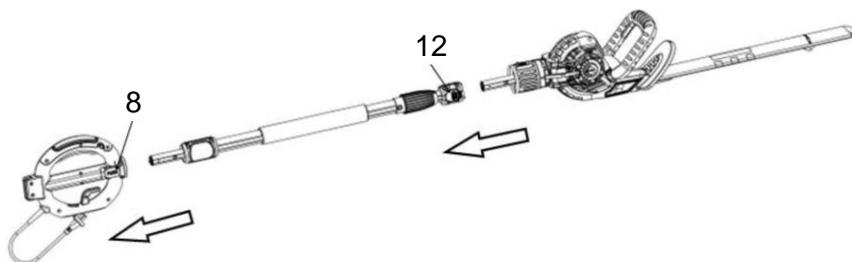
For adjusting the length of the telescopic handle, unscrew the locking nut counter clockwise and pull out the pole up to the desired length. Afterwards re-tighten the locking nut hand-tight.
