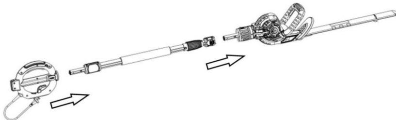
For unlocking and removing the handle from the motor unit, depress the release buttons PUSH on the handle (8) and pull out the handle. To unlock and remove the telescopic handle from the motor unit, depress the release buttons (12) and pull out the telescopic handle.
