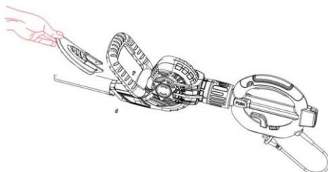
2. Now connect the handle (1) with the motor unit.
