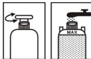
2. Mix concentrates in a separate measuring cup prior to fill into the tank. Add the necessary amount of water and make sure not to overfill the tank. Be careful while mixing, pouring and handling chemicals. The tank capacity is 5 litres.
