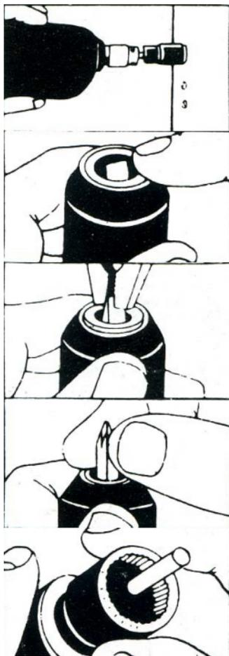
4. Set out and work with constant pressure until screwing complete. When the chosen depth has been reached the screw is released.
